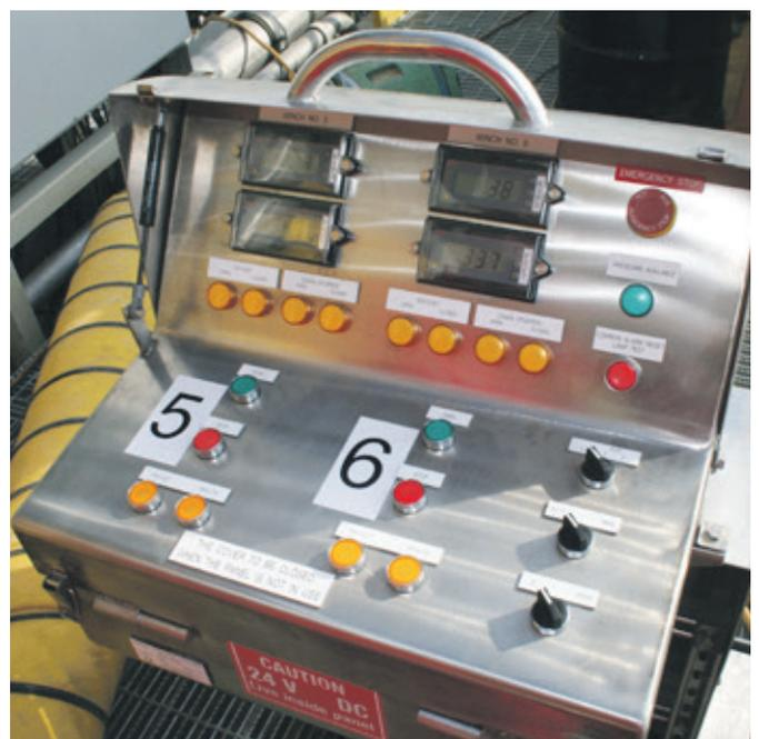
Local control console for operating MacGregor RamWinches on board the *Blind Faith* semi.
