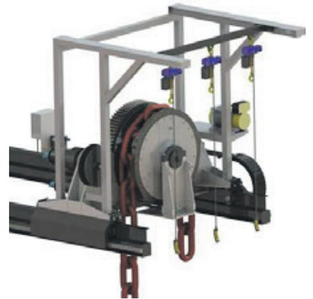
The movable windlass is a concept designed to operate multiple mooring lines within the same area. Normally, one windlass skids along a special foundation to operate one mooring line at a time.
