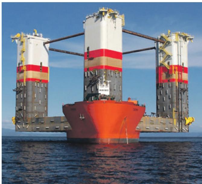
*Blind Faith* semisubmersible being transported to the Gulf of Mexico where it was installed in 2008. MacGregor RamWinches and chain fairleads for 127mm R4S chain were installed at the yard in Norway before sail-away.
