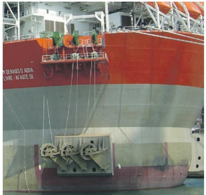
MacGregor eccentric chain fairleads mounted on the hull of BP's Greater *Plutonio* FPSO. The FPSO was installed off the coast of Angola in 2007. This type of fairlead has also been a popular choice for the many spar platforms found in the Gulf of Mexico.
