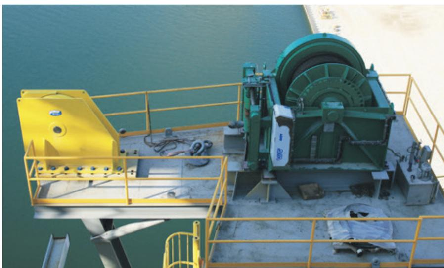
A 100 tonne lateral pull-in winch on board Chevron's *Blind Faith* semi-submersible in the Gulf of Mexico.
