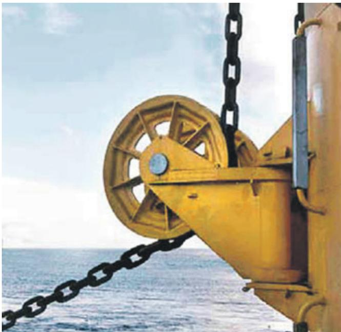
MacGregor eccentric chain fairlead. Fairleads are known for their robustness and they are virtually maintenance-free. Recent designs allow for installation/replacement without the use of a diver. The eccentric chain fairlead has become the preferred choice for both drilling and production vessels. These can also be designed for wire or chain/wire combination. Photo from *Visund* production platform.
