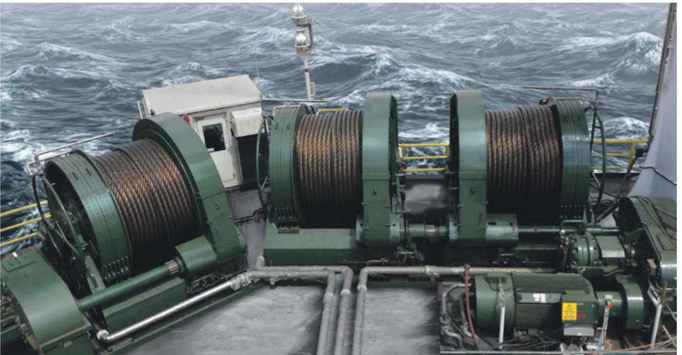
The latest generation of MacGregor mooring winches for the MODU segment is based upon our extensive experience from delivery to more than 50 projects. This experience ensures that safe operation and durability in all climate conditions is reflected in the design. We strive to meet the industry requirement for high stalling power, low equipment weight and low lifecycle cost.
