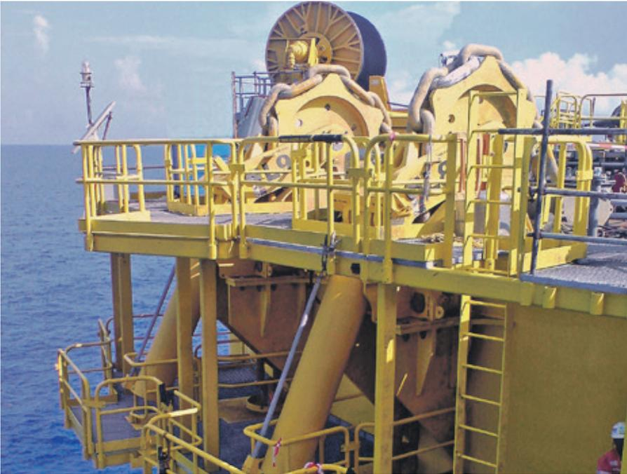
MacGregor Roller RamWinches on board Shells's *Perdido Host Spar*. The nine chain jacks are arranged in three equal groups along the top circumference of the hull. Stalling capacity of each chain jack is 725 tonnes.
