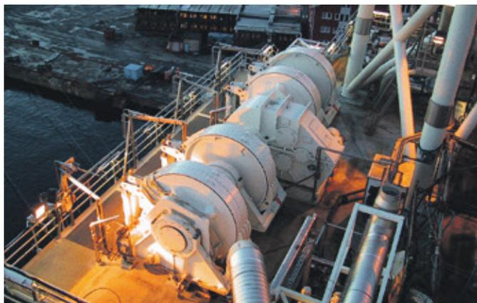
MacGregor anchor windlass for a 145mm chain on board the *Snorre B* production platform in the North Sea. The windlass consists of four cable lifters with a single electric drive/gearbox and two fail-safe band brakes per cable lifter. Brakes can be released using stored energy (accumulator) in an emergency situation.
